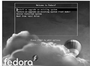
Figure 1-1: Selecting an installation option.
