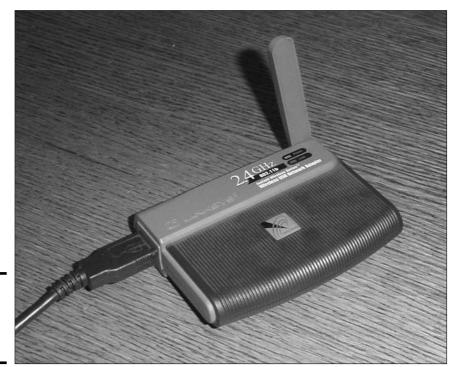
Figure 1-3: A typical wireless networking adapter.
